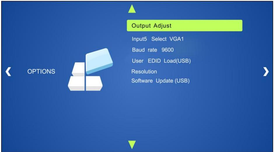
**Output Adjust:** Adjust output image position (X: horizontal direction and Y: vertical direction), ratio aspect (width and height), polarity adjustment (H Polarity and V Polarity) and output setting (HDMI on/off and HDBT on/off).
