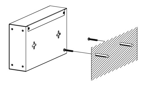
Step 2 – Put 2 screws into the plugs leaving 2mm distance from the wall
