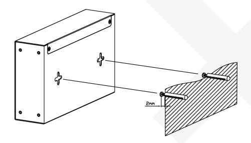
Step 3 – Fit IP09PH in the position corresponding to the screws
