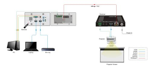
**Note:** We recommend CATx cabling with alien crosstalk prevention technology to ensure the performance of HDBaseT link.
