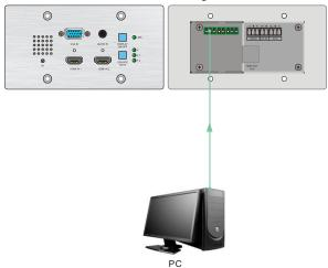
② When control the far-end third party device from local control device (e.g. PC), connect the PC to the RS232 port of the switcher, and then connect the third party device (e.g. projector) to the RS232 port of receiver. The connection diagram shown as below:
