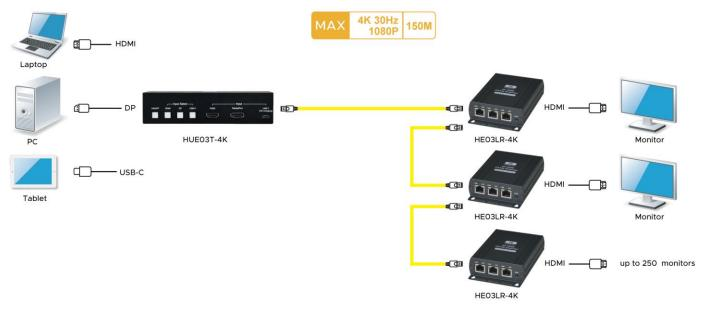
(3) Extends one of HDMI/DP/USB-C signals to multiple displays through Gigabit Ethernet Switch
