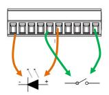
Please check the positive and negative of LED before connect the cable. Otherwise, it might damage the device or lead no reaction.
