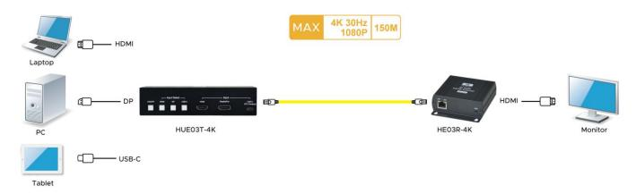
(2) Extends one of HDMI/DP/USB-C signals to multiple displays
