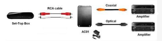
b. Digital input convert to Analog output:
