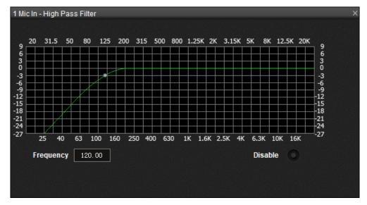
3. Users can choose cut-off frequency of High-Pass Filter, 120Hz for recommendation.
