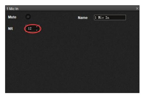
4. The parameters of Noise Reduction have 0, 6~18, total 14 choices. 0 represents NR algorithm closed; 6 represents NR ratio 6dB; 18 represents NR ratio 18dB; 12dB for recommendation, see the red circle above.
