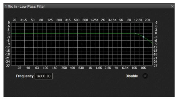
3. Users can choose cut-off frequency of Low-Pass Filter, 16000Hz for recommendation.
