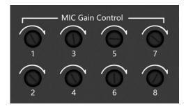
When you adjust the Gain, you can use a "one" screwdriver to turn up in clockwise direction, and turn down in counterclockwise direction.
