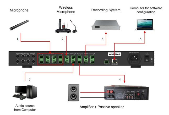
Devices will be connected through the interfaces in the rear panel, details are below.
