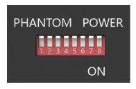
The DIP switch downward means that the phantom power supply "on" of the corresponding microphone, and upward means the phantom power supply "off". Normally the phantom power supply remains "on" status.
