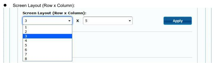
Set up the number of vertical and horizontal monitor based on the video wall layout. Vertical number 1~8 and horizontal number 1~16.
