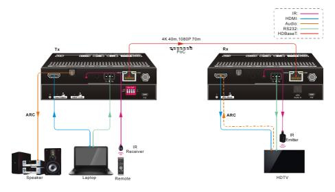
**Note:** The STP cable is recommended to be used to ensure optimal machine performance in ARC mode.
