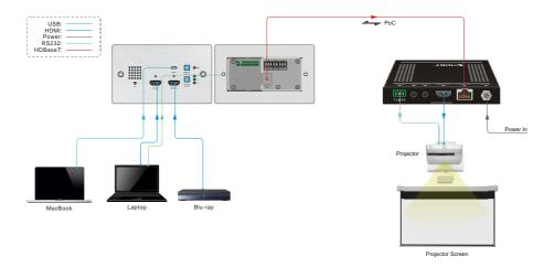
**Note:** We recommend CATx cabling with alien crosstalk prevention technology to ensure the performance of HDBaseT link.
