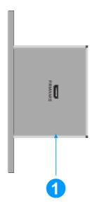
① **FIRMWARE:** Micro-USB port for firmware upgrade.
