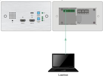
When control the far-end third party device from local control device (e.g. PC), connect the PC to the RS232 port of the switcher, and then connect the third party device (e.g. projector) to the RS232 port of receiver. The connection diagram shown as below:
