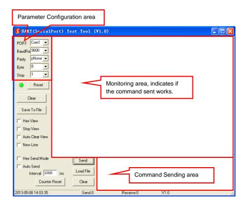
Please set the parameters of COM number, bound rate, data bit, stop bit and the parity bit correctly, and then you are able to send command in Command Sending Area.
