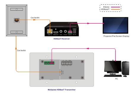
② Control the TPUH406T-EU by the remote PC which is connected with Receiver.
