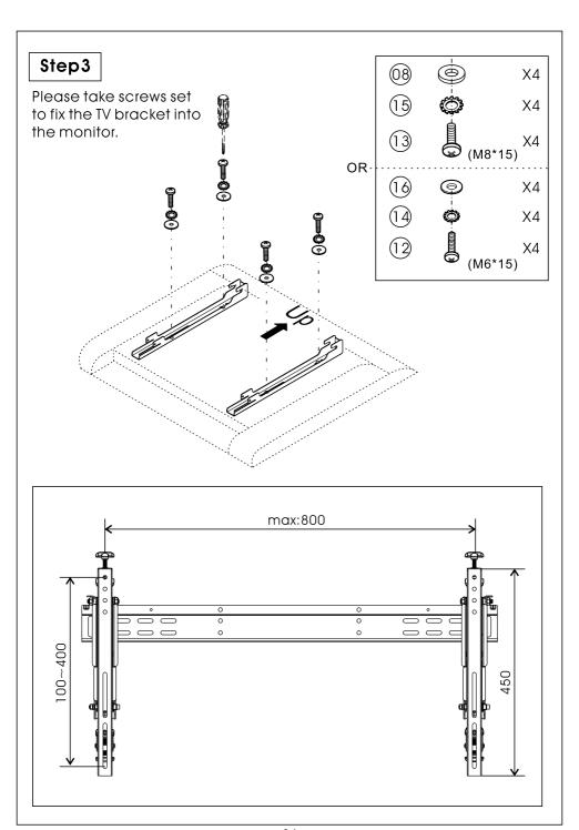
After finish the step3, please go to fix the monitor into the bracket and complete to assemble the TV bracket as figure.
