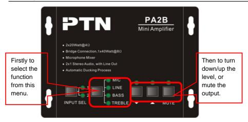
For example, to turn up the line volume, you should select the "LINE" first, and then press the button "...".
