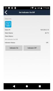
Touch Indicator On, the power LED of host will keep flashing and show OSD message "I am here" on monitor
