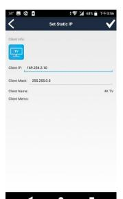
Enter IP address and subnet mask then touch top right  $\lceil \mathbf{V} \rfloor$  button to finish setting
