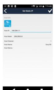
Enter IP address and subnet mask then touch top right  $\lceil \mathbf{V} \rfloor$  button to finish setting
