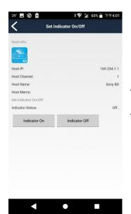
Touch Indicator On, the power LED of host will keep flashing
