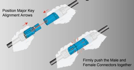
Rotate the Male and Female connectors in opposite directions until the Padlock symbol is in alignment with the Arrow symbol
