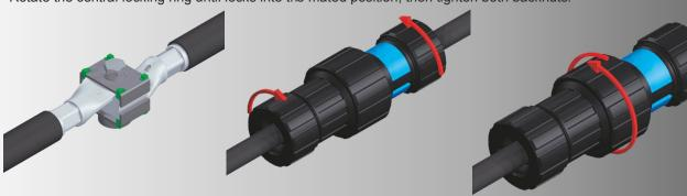
Lock the Central Locking Ring using the remote locking / release key.
