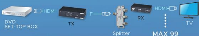
One TX to Multiple RX Connection (with splitter)
