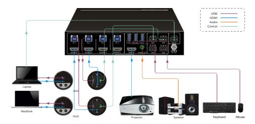
The switcher is used with four SC-GRHU table grommets:
